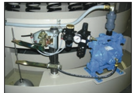
Machine Discharge Lift Station —Transfers discharged compound and water to waste treatment or recirculation system.
